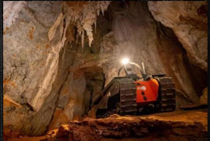
The TerrusM is based on the CatPack, as seen here on a CSIRO Data61 robot in the DARPA SubT Challenge
